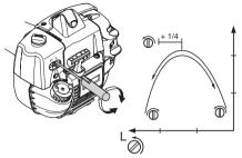
**CAUTION!** If the cutting attachment rotates when the engine is idling the idle adjustment screw T should be turned anti-clockwise until the cutting attachment stops.
